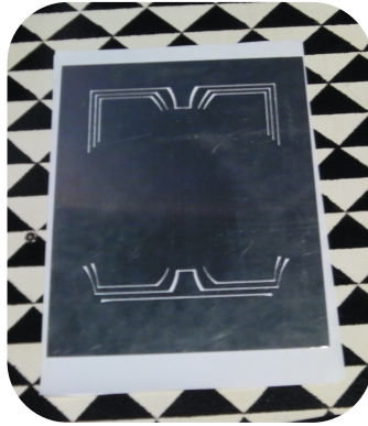
FIGURE 11. WATERJET CUT ALUMINUM DRY EMBOSSEING PLATE, 20 x 25 CM, JULY 2011, DIGITAL DOCUMENTATION.
