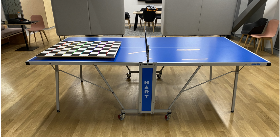
Figure 3.7. Finding the corners of a chessboard in an image for camera calibration
