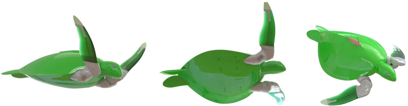
Figure 21: Final sea turtle robot design based on the green sea turtle ( Chelonia mydas ).
