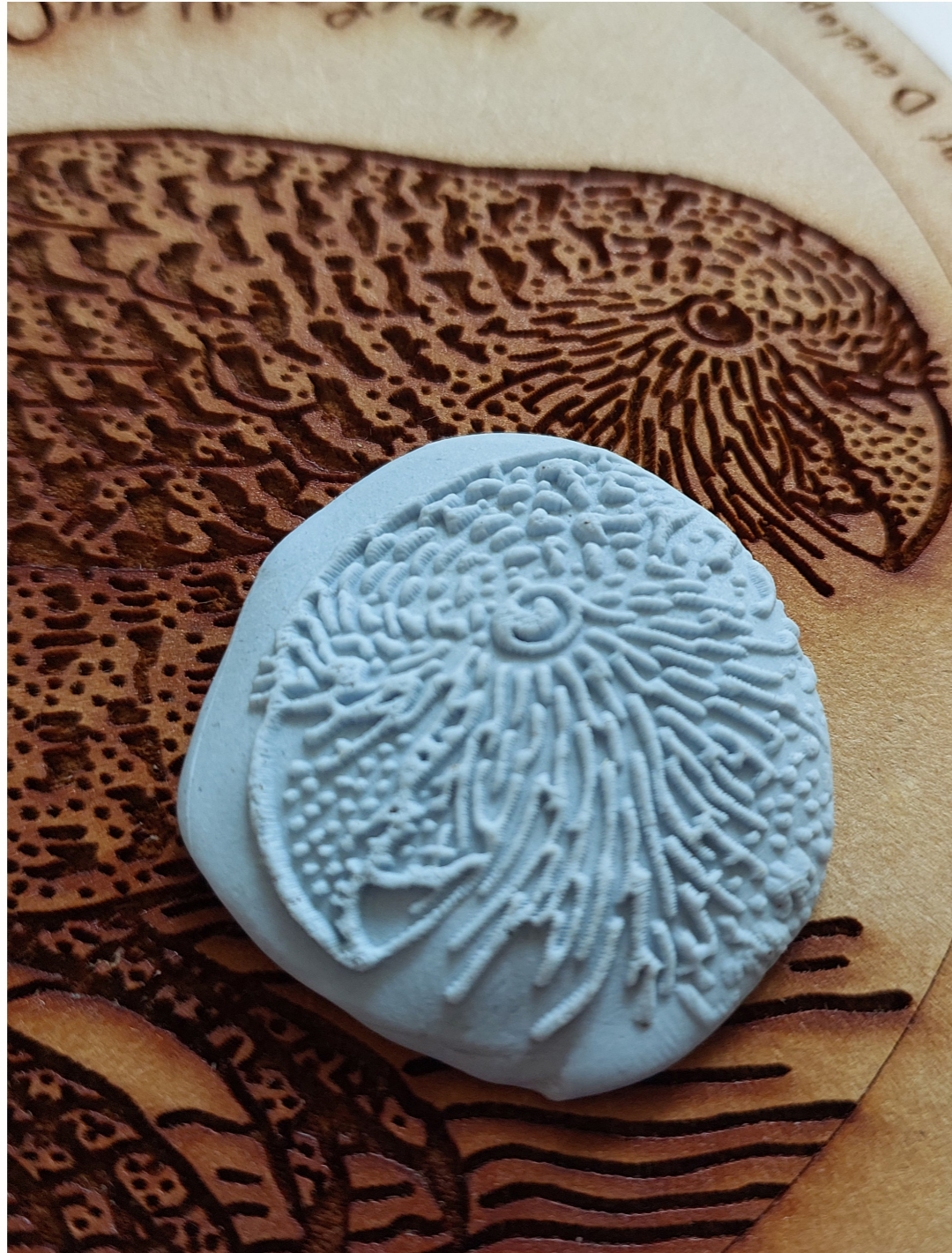
Figure 89. Up close of the The Kākāpō token lasercut on mdf (front) and the relief the engraving leaves on putty
