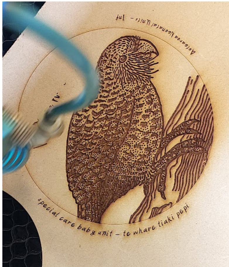
Figure 83. The Kākāpō token being lasercut on MDF (front)
