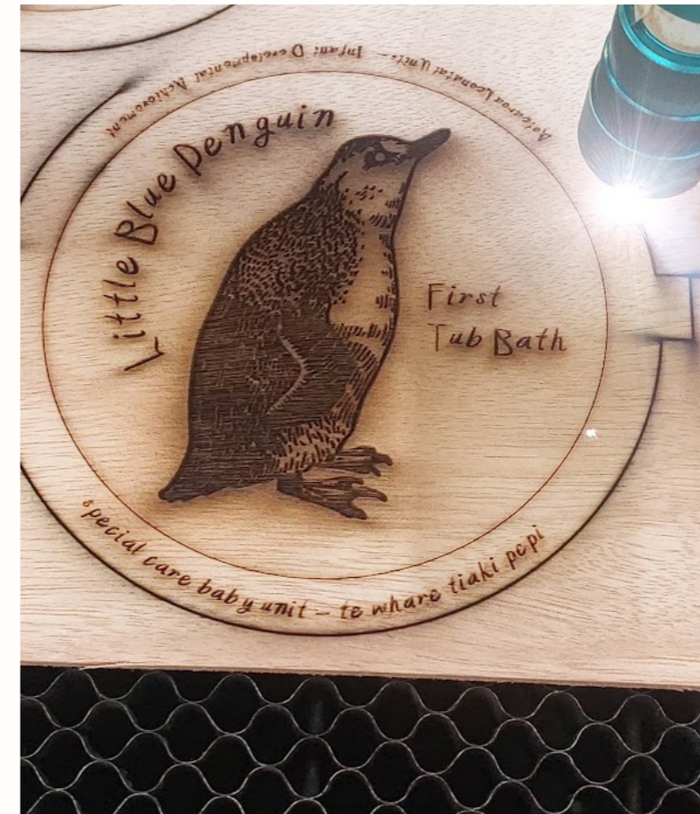
Figure 85. The Little Blue Penguin token being lasercut on 2mm plywood (front)
