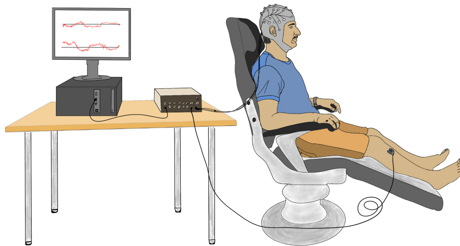
Figure 4.3: An illustration of the laboratory setup for recording of EEG and sEMG data
