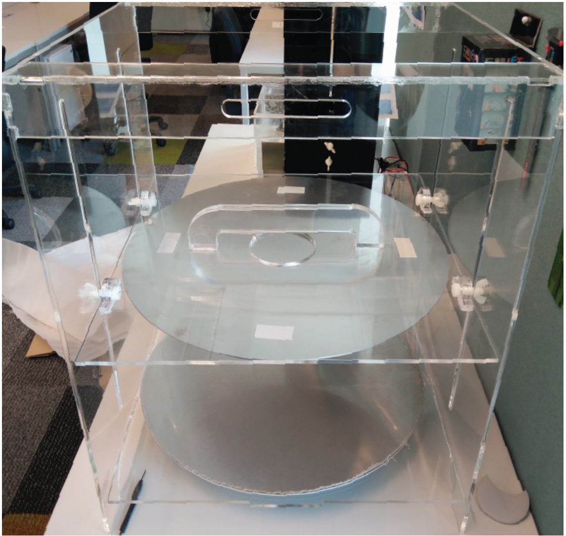
Figure C.2: Capacitor Box Setup – Complete Build with Two Round Plate Electrodes
