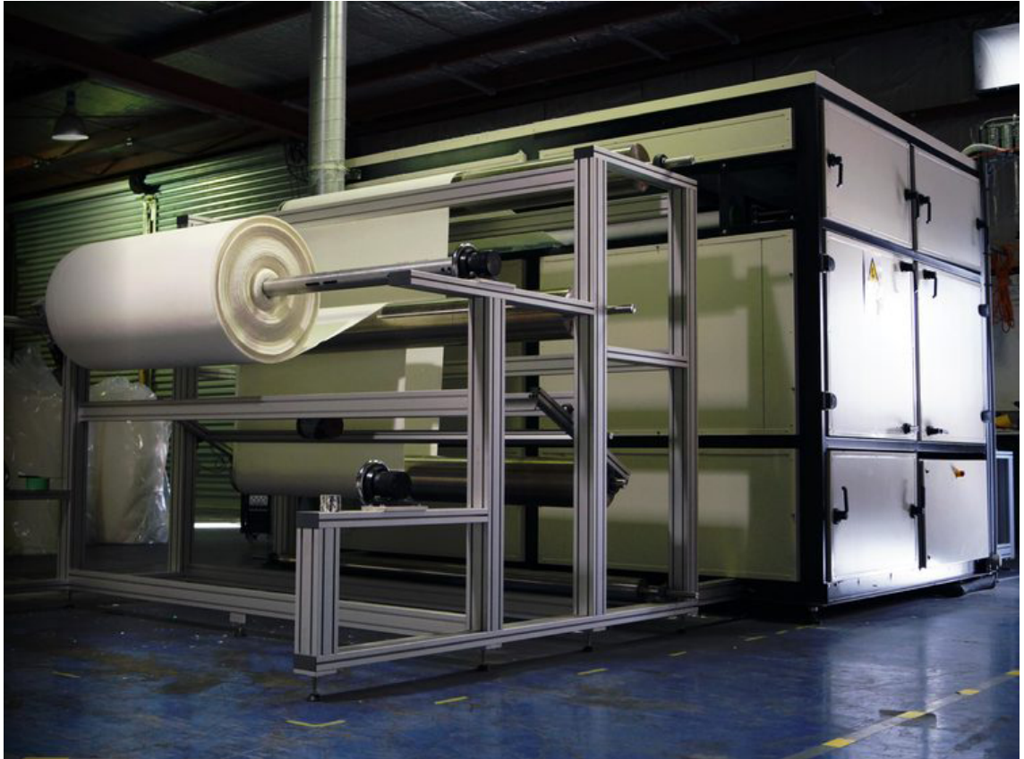
Figure 1.1: Revolution Fibres production scale adaptable nanofibre manufacturing machine named 'The Komodo' – Image courtesy of Revolution Fibres
