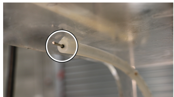
(b) Tinned end of the HVDC lead
