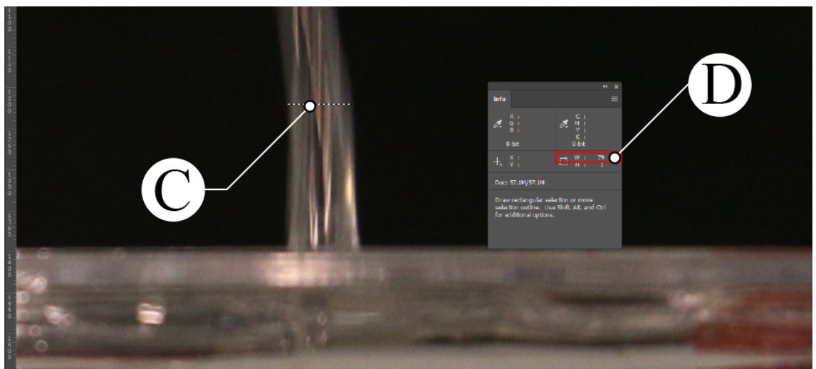
(c) Measuring diameter of jet in pixels (C) and recording count (D)
