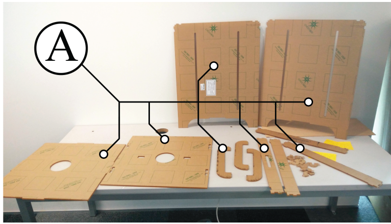
(a) Laser Cut Perspex (A) shown with protective brown sticker
