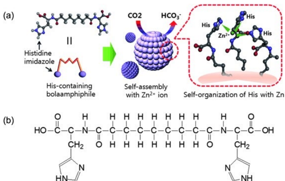
Figure 3.5. a) Schematic representation of the hydration process of CO 2 through the self-assembly of the histidyl bolaamphiphilic molecule (His-C 7 ), which stimulates the active site of carbonic anhydrase, and b) chemical structure of His-C 7 (His = Histidine). Source: Reprinted with permission from ref. 148. Copyright (2013) Chemical Reviews.
