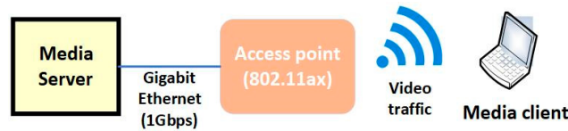
Figure 1. Test-bed for an 802.11ax infrastructure client–server network.
