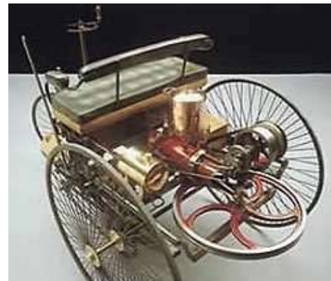
Four-stroke IC engine powered automobile 1885
