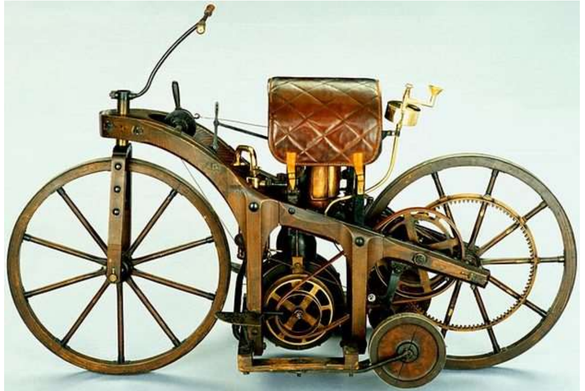
Four-stroke 0.5HP IC engine powered motorcycle 1885
