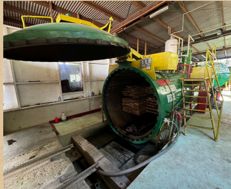
Figure 4.1.4. A timber treatment plant at LTD Wailevu, Labasa (photo by the author).
