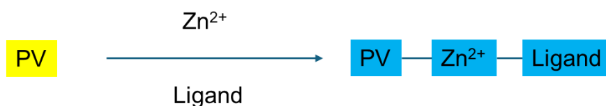
Figure 63: Colour change of PV from yellow to blue upon complexation with Zn^{2+} .
