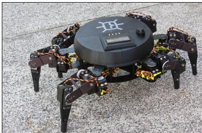
Fig. 4-33 ANN Implemented on Hexapod Robot
