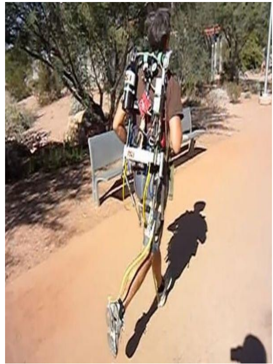
Figure 13: Jason Kerestes of Arizona State University has developed an exoskeleton with the help of DARPA that allows its operator to run 10% faster than (s)he usually can (Farrier, 2014).
