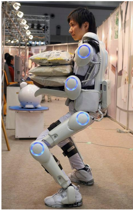
Figure 12: A robotic Suit developed by the University of Tsukuba that allows its operator to carry heavy loads easier (Kamoshida, 2005).
