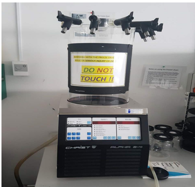
Figure 6. It is the Freeze dryer
