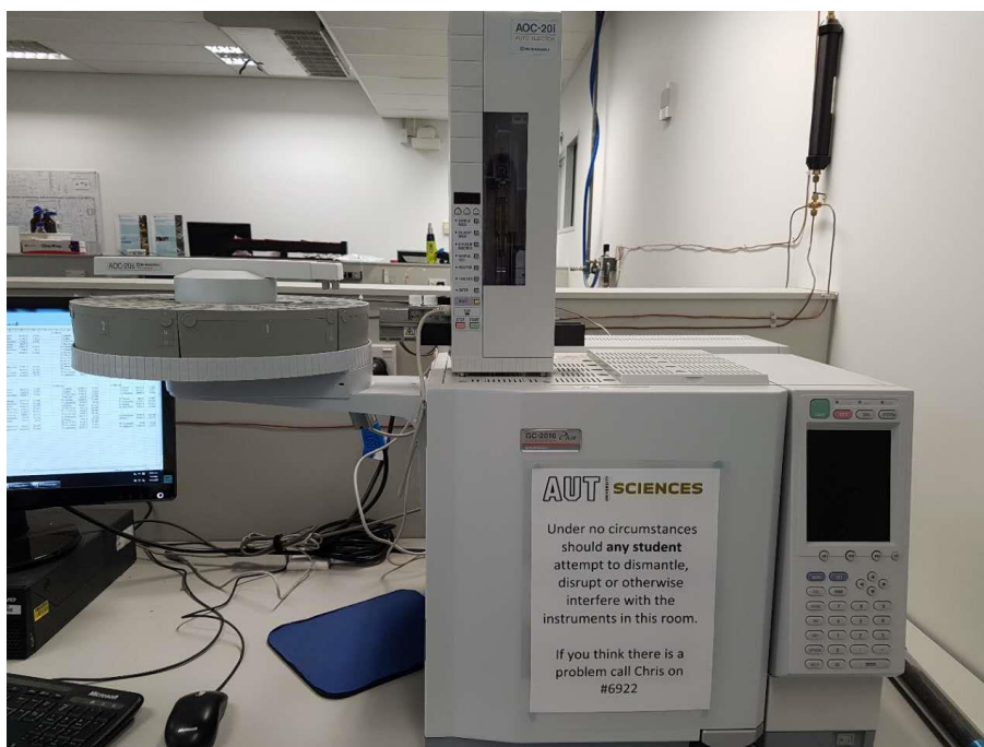
Figure 7. Shimadzu GC2010 gas chromatograph used in this study equipped with a Flame Ionisation Detector.
