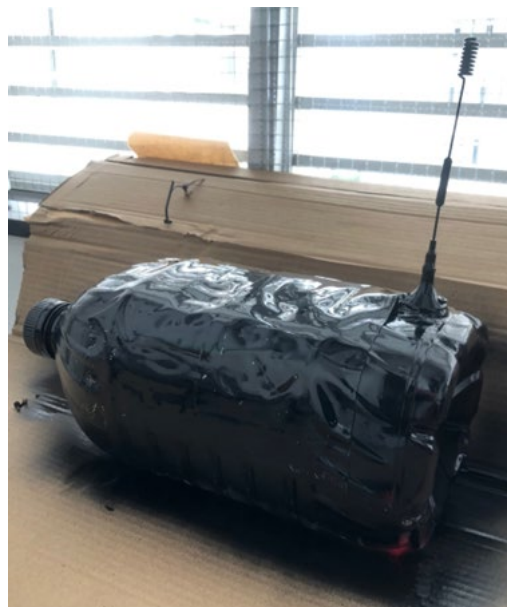
Figure 4: (Cleveland, 2022) Plastic Tracker final prototype as released into the river [photo].
