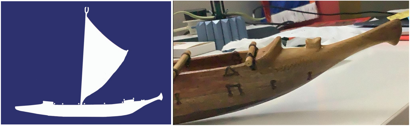
Figure 15: Illustration of sailing vaka and image of model vaka highlighting 'te yiku ote mango'
