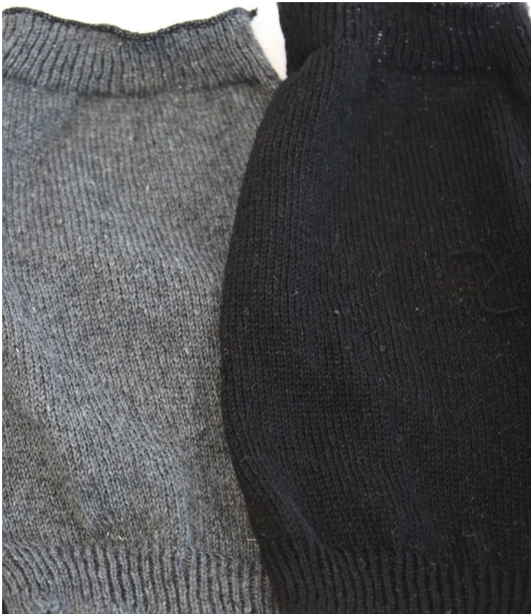
Figure 57: Swatches knitted on the Shima Seiki using the grey and black 1/150 tex yarn.
