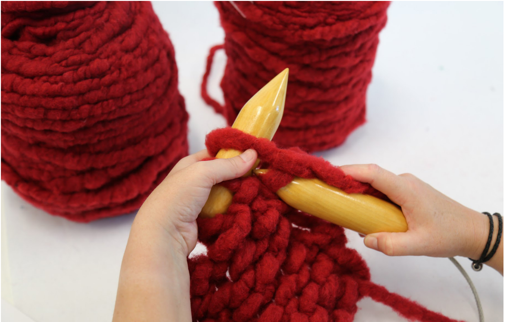
Figure 61: The red core spun yarn was handknitted using a very large 35-millimetre diameter circular needle.
