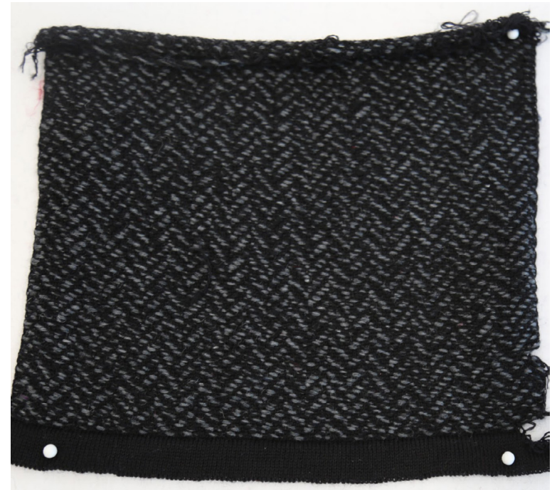
Figure 60: Swatch knitted on the Shima Seiki SRY 123 LP inlay machine, using the black 1/150 tex yarn the coarser 2/150 tex black and grey yarn.
