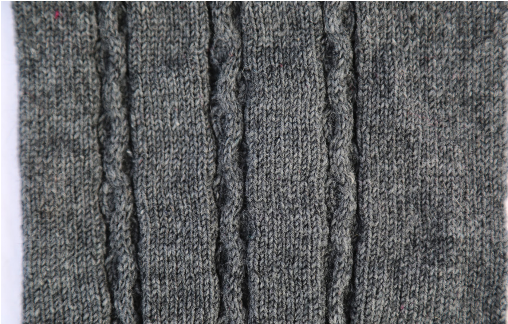
Figure 59: Swatch knitted on the Shima Seiki using a cable pattern.
