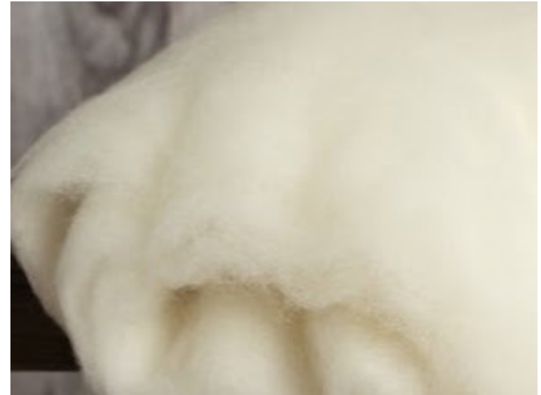
Figure 63: In comparison the wool batts are also directionally aligned within the batts.
