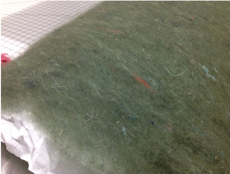
Figure 62: The fibres were directionally aligned within the batts and the fibres seemed to hold together into a sheet.
