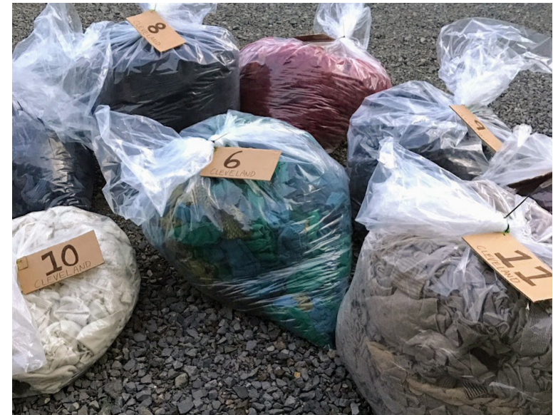
Figure 55: The colourways were packaged and labelled so that the textile waste was introduced into the shredder and opener as a procession.
