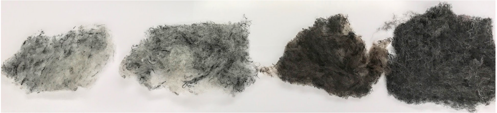
Figure 40: Different percentages of the recycled textile waste were combined with virgin wool and hand carded and felted into samples.
