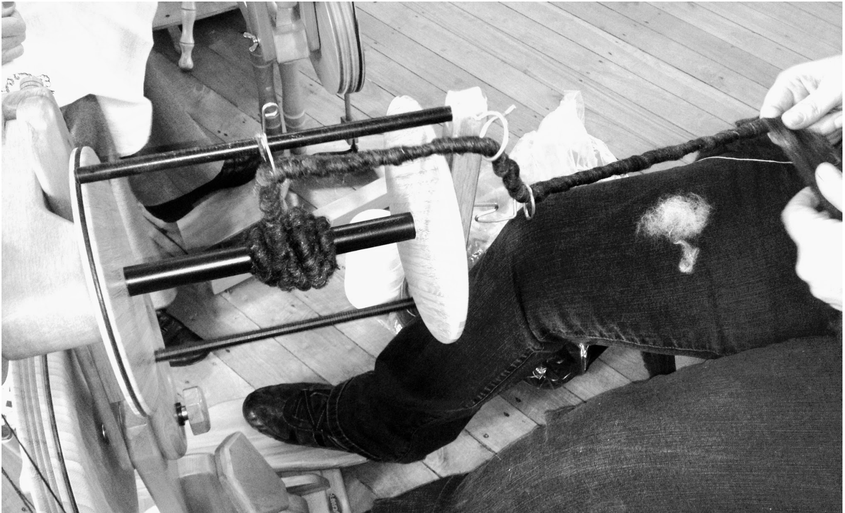
Figure 51: To test the viability of the core spinning process samples were first developed by hand.
