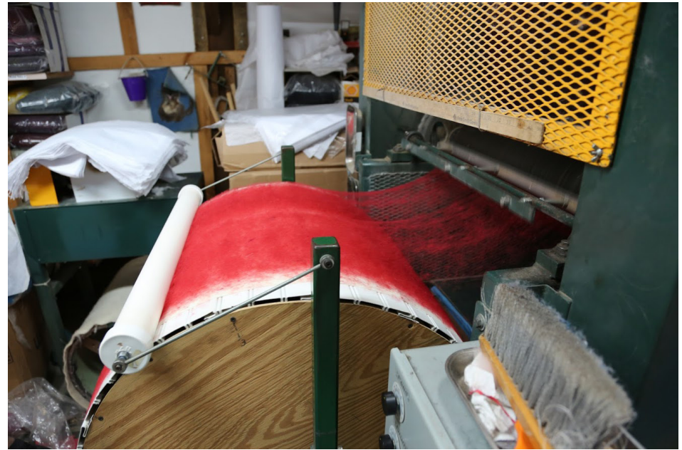
Figure 38: The fibres being drawn off into a batt on the back of the Stone Hedge Carder.
