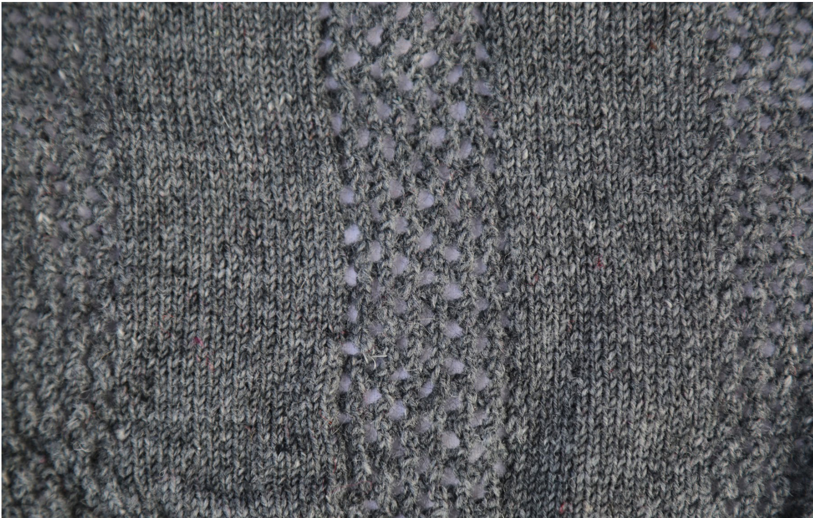
Figure 58: Swatch knitted on the Shima Seiki using a lace pattern.
