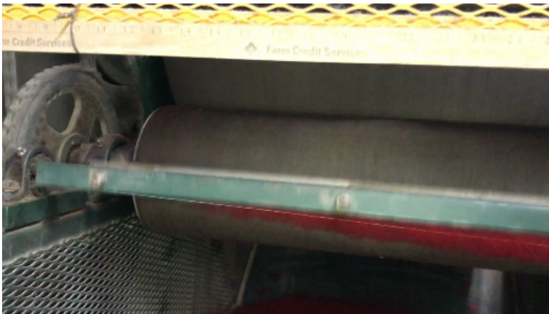
Figure 53: Fibres being drawn straight from the carding machine and wrapped around a core as they exit the carding machine.
