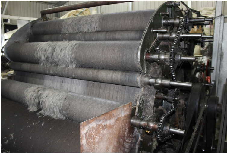
Figure 36: The Haign Carding machine has many cylindrical rollers that work at different speeds and in different directions to open the fibres and align them as they pass over.
