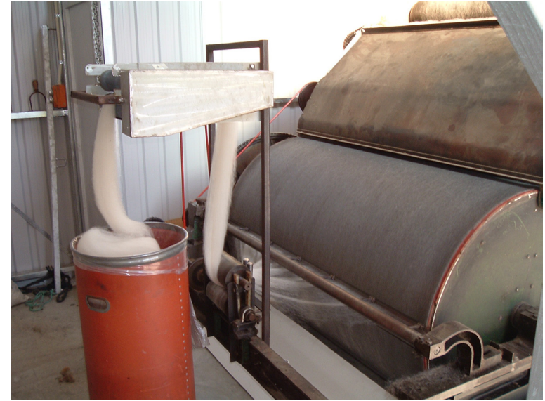
Figure 37: Fibres being drawn off the Haign Carder in a sliver.
