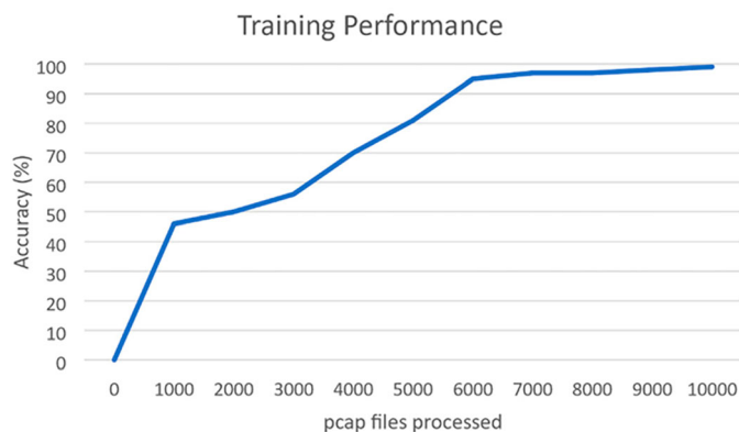
Figure 4. CNN training accuracy rates per PCAP file.
