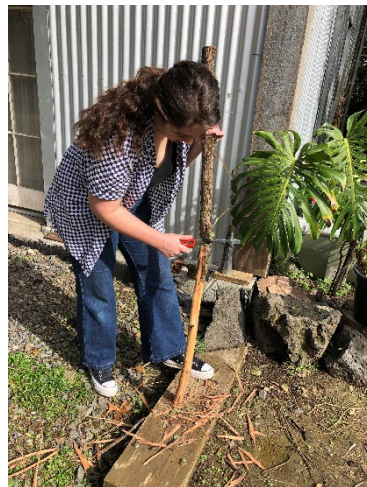
Figure 8 Hewing a kānuka strongback, freshly harvested from the grove. May 3, 2024, Woodhill Farm.
