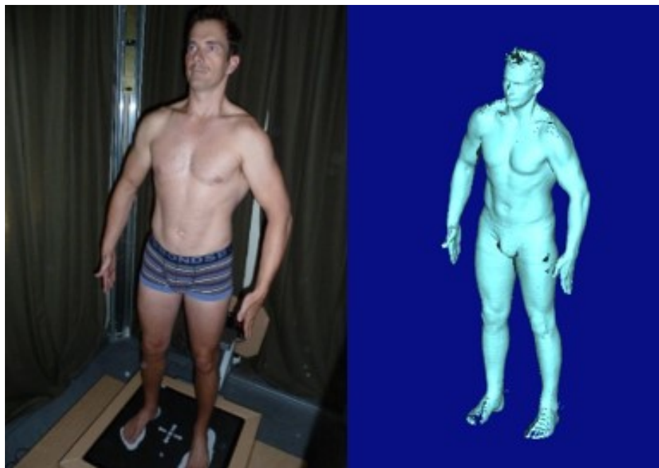
Figure 3—4. An example of a scan posture within the Vitus XXL. Body postures vary from participant to participant and if not controlled, is a potential source of measurement error.
