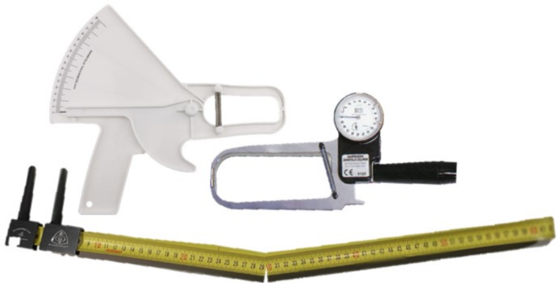
Figure 2—5. Differences in Harpenden and Slim guide skinfold callipers and an example of a broken segmometer.
