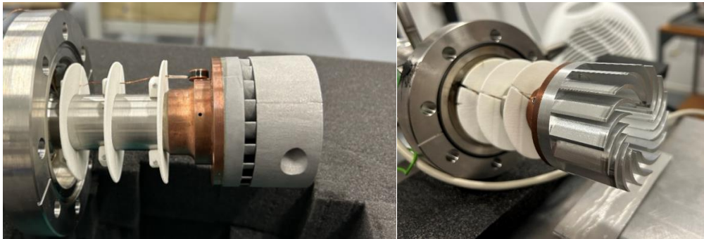
Figure 4. Left, the original 3D printed heat exchanger, and right the new heat exchanger with increased heat transfer area. Both mounted on the cryocooler.
