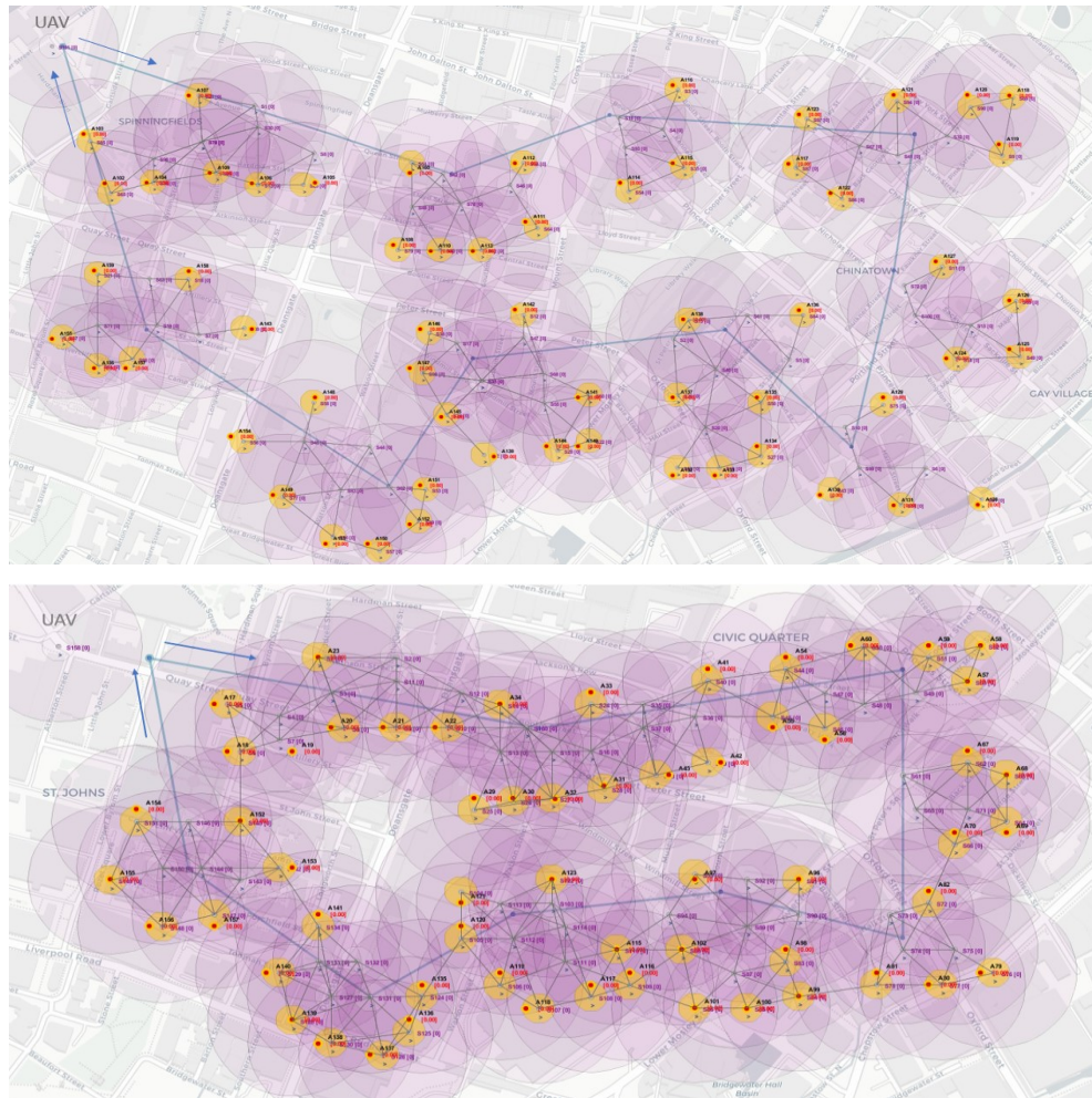
Figure 5-15 Data gathering of grouping sensor nodes designed in CubCarbon (upper design belongs to the sparse network with \sigma_{gc}=750 , while the lower one belongs to dense network with \sigma_{gc}=250 ).
