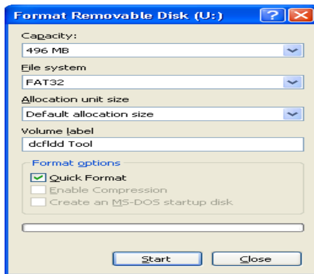
Figure A11. 8: Formatting the sterilized USB drive with FAT 32 after wiping (Step 7)
