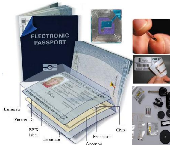
Figure 2.3: RFID Tags (adapted from: www.uktelematicsonline.co.uk ; www.electronics-lab.com ; www.associatedcontent.com ; www.media.photobucket.com ; www.prisms.cs.umass.edu )
