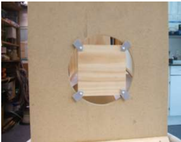
Figure 4.4 Sample holder for the angle of depolarisation experiment
