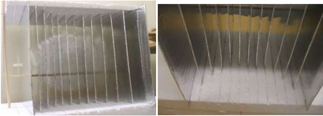
Figure 2.12 Implemented metal plate lens
