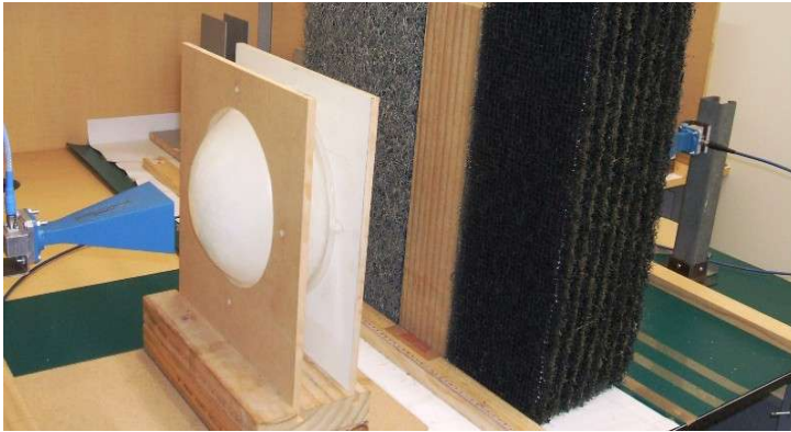
Figure 4.15 Implemented transmission coefficient measurement setup
