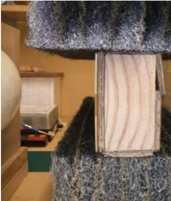
Figure 5.3 Position of the sample for reduction of diffraction from the sample edges
