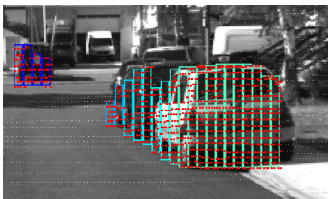
Figure 3.19: Extracted stixels (colour-coded by depth) and LiDAR points marked by white and red dots. Points hitting any extracted stixel are shown in red and used to evaluate the accuracy of the extraction process.
