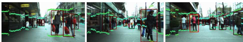
Figure 2.13: Pedestrian-based stixel estimation; green lines indicate stixels [14].
