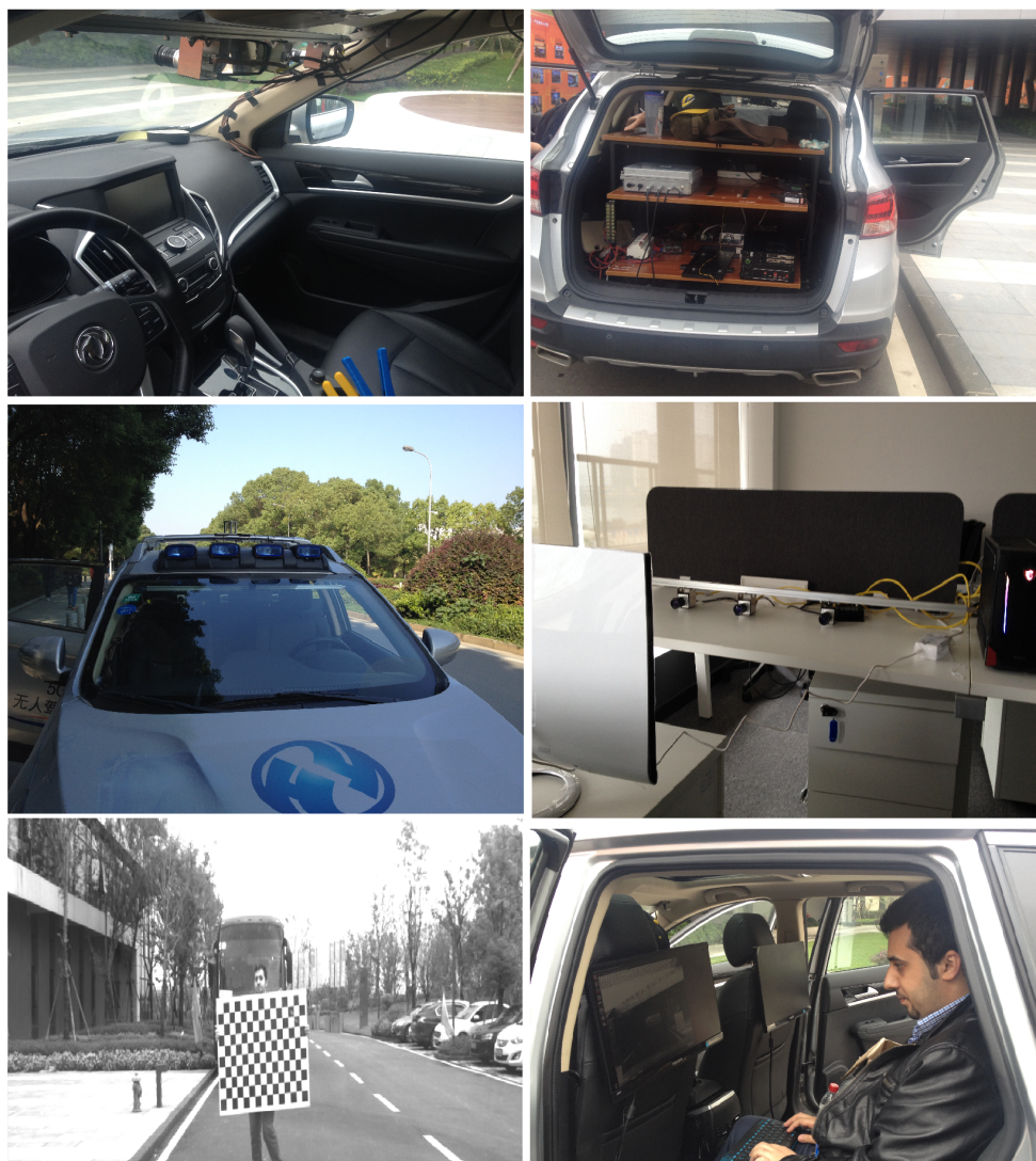
Figure 1.5: Trinocular vision configuration. Test vehicle, as used while at Wuhan University in October 2016
