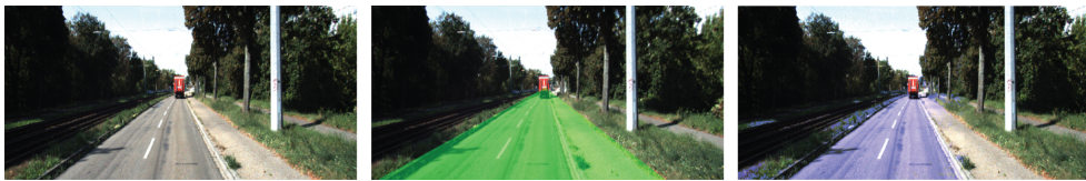
Figure A.1: Comparison of free-space detection results. Left : Original image. Middle : Free-space using monocular detection, as estimated in this paper. Right : Free-space using binocular vision, as used in this paper. Green is used for the monocular, and purple for the binocular vision case.
