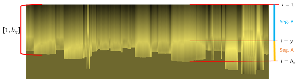
Figure 4.4: Benefit image, where bright pixels present perfect cut between background and foreground.
