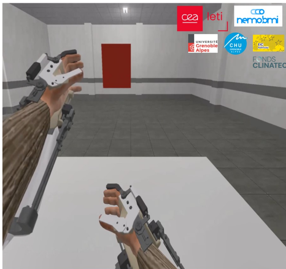
Figure 4. Experimental set-up for 6DoF DB acquisition. The patient is asked to control the virtual avatar with 6 degrees of freedom to move his left or right hand or to stay idle. Both hands trajectories are described by sequence of target positions defined by their coordinates in 3D space.
