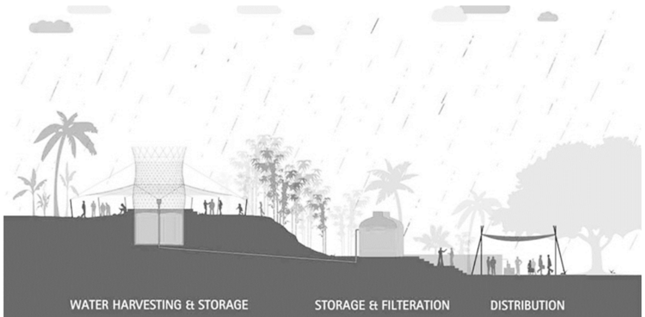
Figure 29. © Warka Water. Meshed fabric to collect rainwater diagram, drawing/ digital, 2015.
