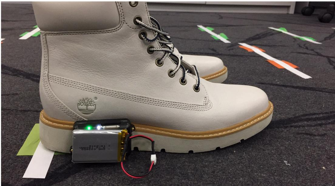
Figure 4.5: IMU attached to boot
