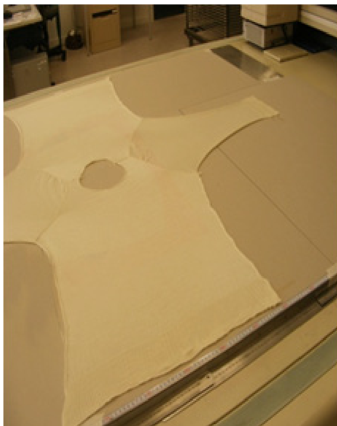
Fig2:25 (Above) This image shows the garment half assembled ready for the printing process. The print has been designed in such a way so that the print will continue across the shoulder seam to the back of the garment. The print orientation is an important consideration when making prints for the front and back of the garment
