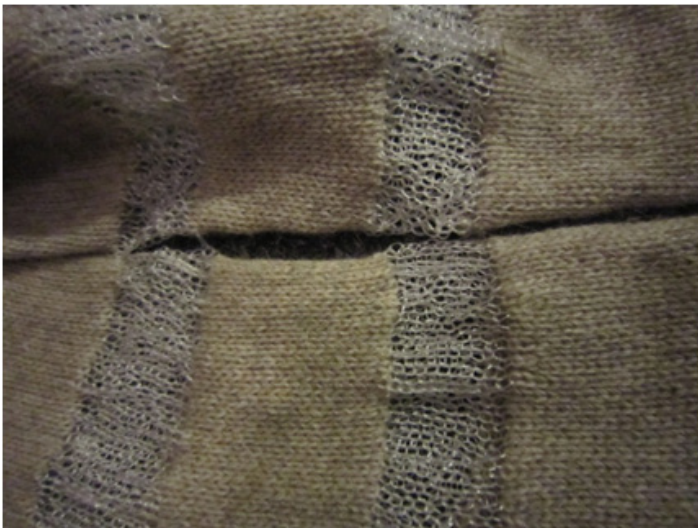
Fig 3:38 (above) & Fig 3:39 (below) Shows the stripes on the body of the garment lining up correctly with the sleeve stripes. This is technical as well as aesthetic, as when the hands are rested by the side, the stripes will align. Once the stripes have been correctly programmed, then the inclusion of the structure design can be used.
