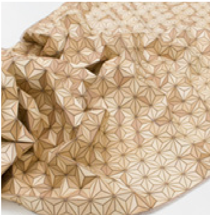
Fig 1:23 Strozyk's fabric- like rugs are using solid materials which are cut cut in such a way to act as a textile fibre would.
