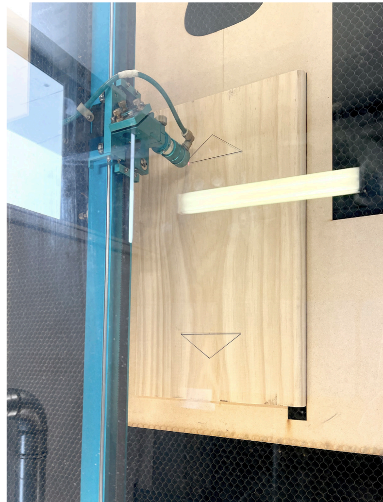
Figure 52. Laser cutting hand-holding part.
