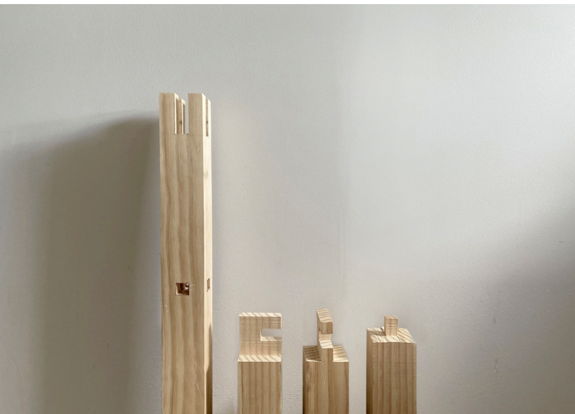
Figure 60. The structure experiment of wood-joint connection.
