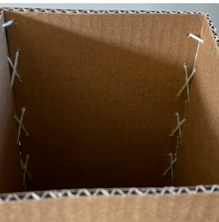
Figure 35-36. Cardboard material prototype making, Connection version 1.
