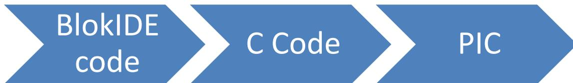
**Figure 6 BlokIDE to PIC process**
