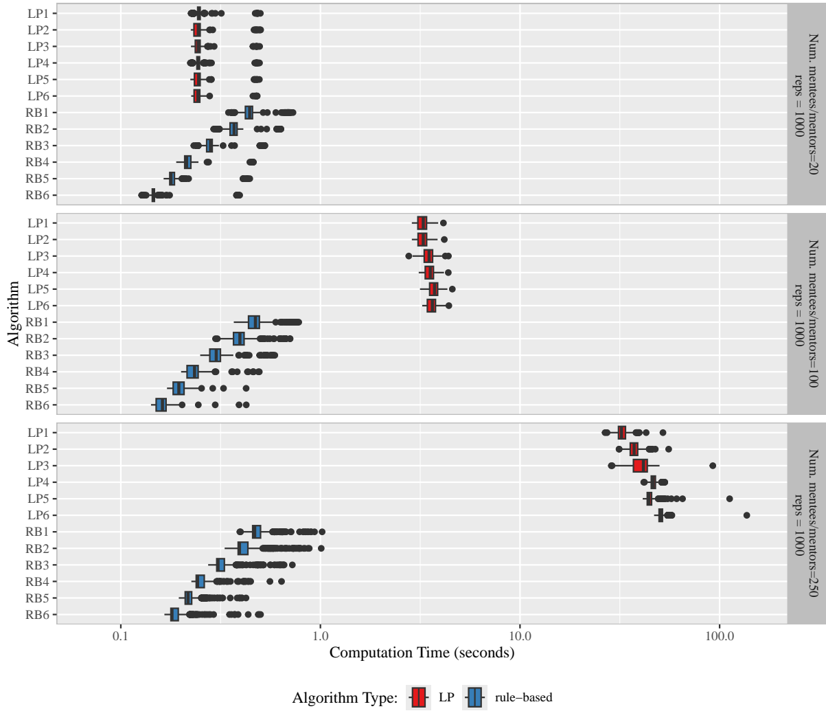
Figure 5: Distribution of computation time to run algorithms for 1000 cohorts of mentees (randomly generated from mentee scenario 1) and mentors (randomly generated from mentor scenario 1). Times in seconds are presented on a log scale.
