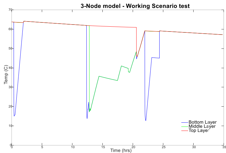
Fig. 53. Example of the output generated by a three-node moving boundary model and an Euler marching scheme. The output of this model was disappointing and did not improve on the simulated output of the two-node stratified model.
