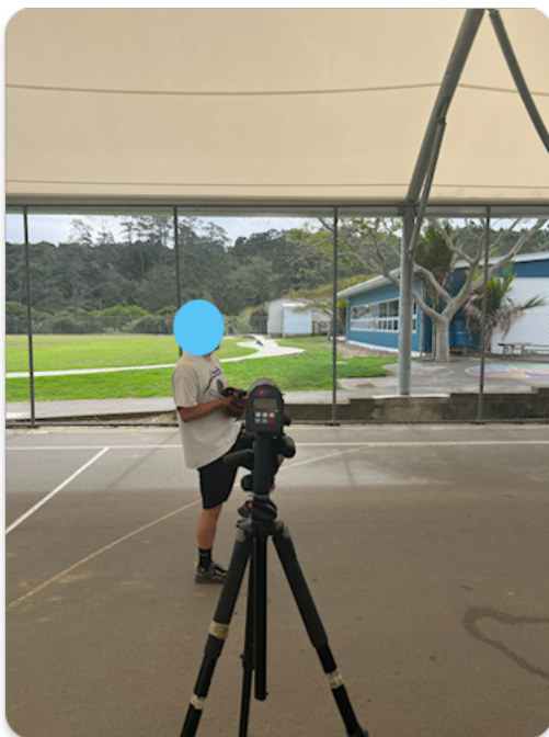
Figure 6. Set-up from behind radar gun showing data collection view
