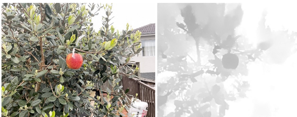
Figure 4.1: An example capture taken of an apple 0.5m away from the camera origin. The Depth map (right image) represents all LiDAR data per pixel gained from the IOS device.
