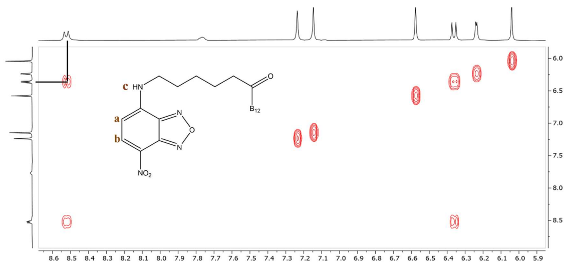
Figure 35: Aromatic region of the COSY spectra of 3 obtained in \text{MeOH-}d_4 , highlighting the correlation for the NBD-X protons at 6.36 (1H, a ) and 8.52 (1H, b ) ppm.
