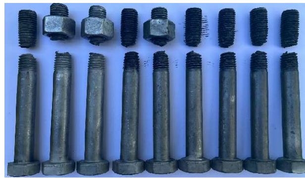
Figure 8 Failure modes of the group GA 50 lubricant.
