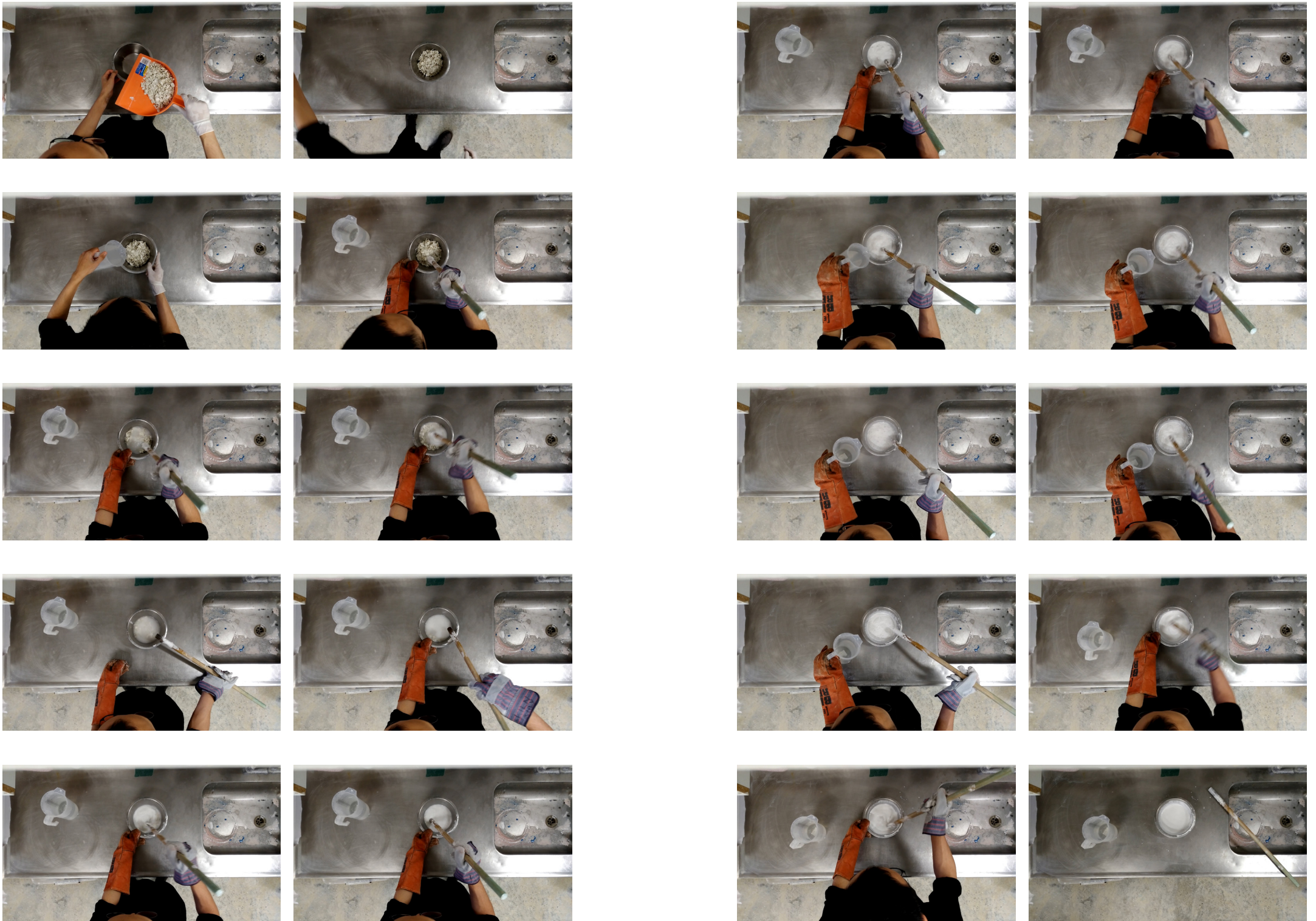
Figure 73. Stills from video of batch slaking quicklime from fired shells.
