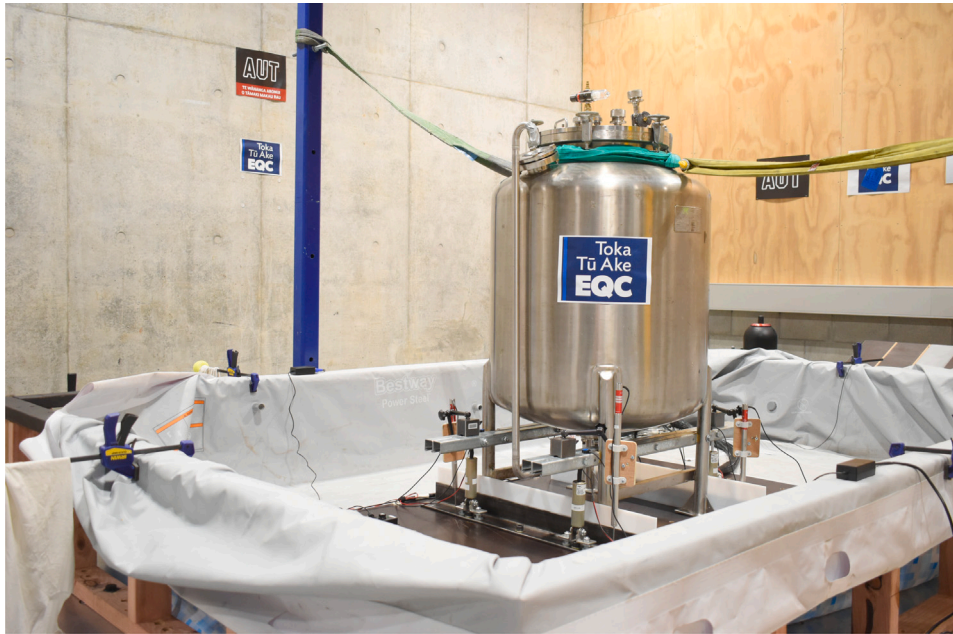
Fig. 5. Experimental setup of the tank with MR dampers.
