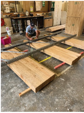
(a) Mounting columns (poupou) onto backing frames in UoA architectural laboratory
