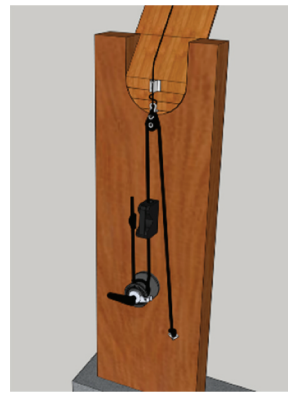
(b) Rendered view of live end and clutch
