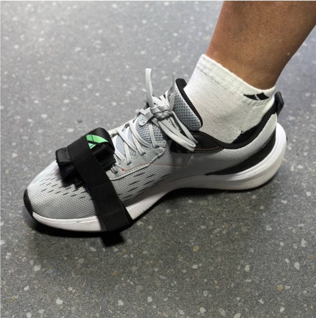
Figure 29. Attachment of the IMU sensor to the shoe using a Velcro strap
