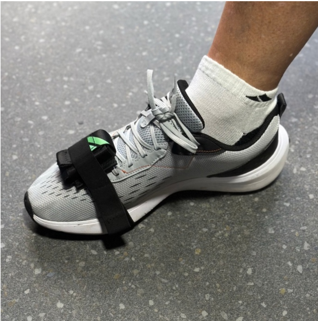
Figure 21. Attachment of the IMU sensor to the shoe using a Velcro strap
