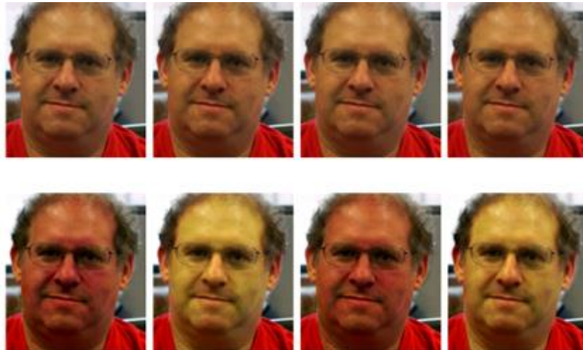
Figure 3.7 Colour Variation Magnification: Input frames (top) and Magnified frames (bottom) [30]
