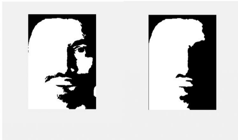
Figure 5.10 Logical Operation and Image dilation (left) Polygon to Region mask (right)
