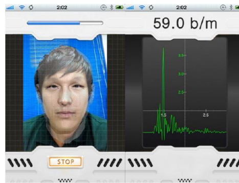
Figure 3.2 FaceBEAT: supports overlaid guide view on the recording(left) estimated heart rate and the FFT results (right) [97]
