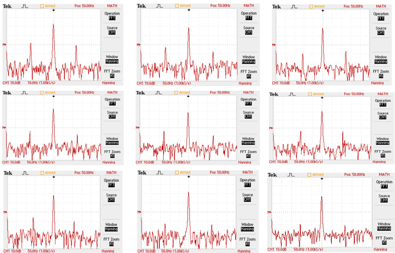
Figure 15. Individual FFT spectrum analysis of electric Motor 1–9 without load.
