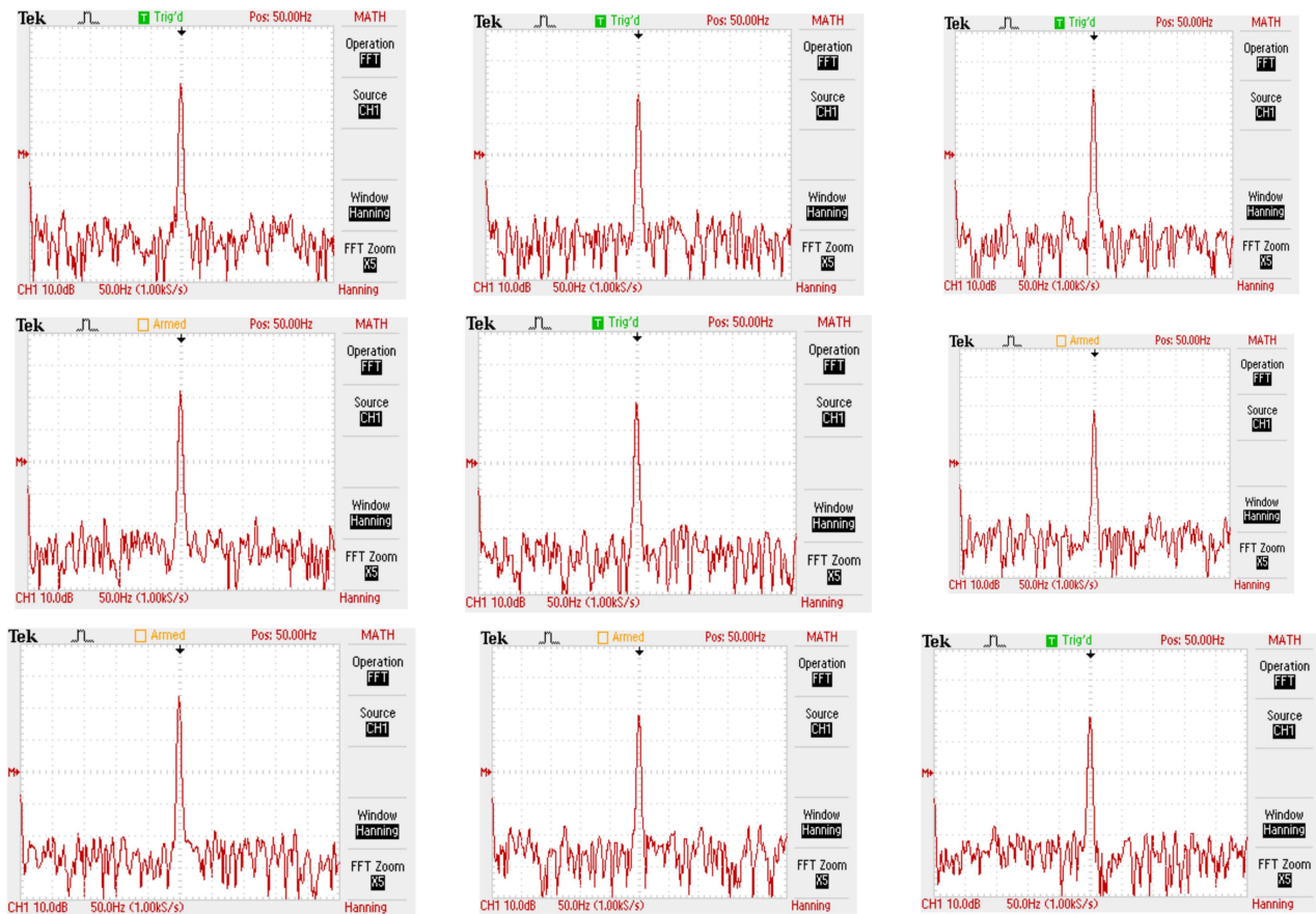
Figure 14. Individual FFT spectrum of electric Motor 1–9 without load.
