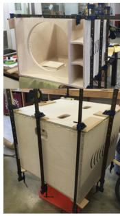
Figure 33: Building the first subwoofer in the 3DLab workshop, AUT University.
