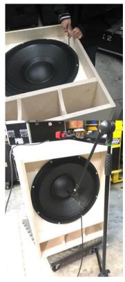
Figure 34: Testing how low the 21" sub can go - the resulting 32Hz resonance is lower than most!
