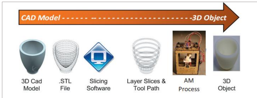
Fig. 2.8 Schematic of additive manufacturing process (Azlin et al., 2022)
