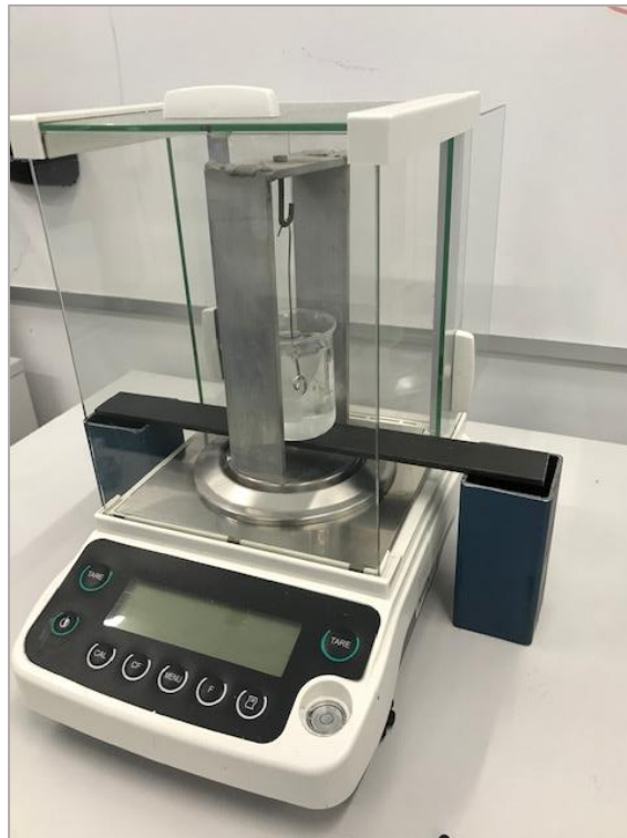
Fig. 3.16 Archimedes Density Measurement Experimental Setup
