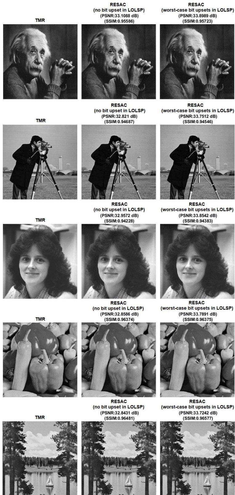
Fig. 3. Digital images processed using TMR and RESAC. In RESAC, no bit upset and worst-case bit upsets in LOLSP (which is unprotected) are considered.
