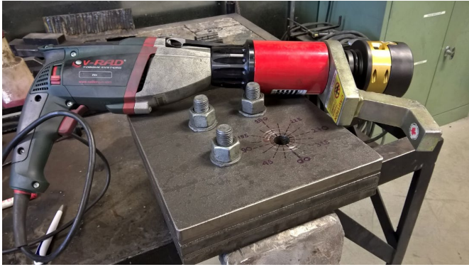
Figure 1 Bolt tightening test setup and torque multiplier
