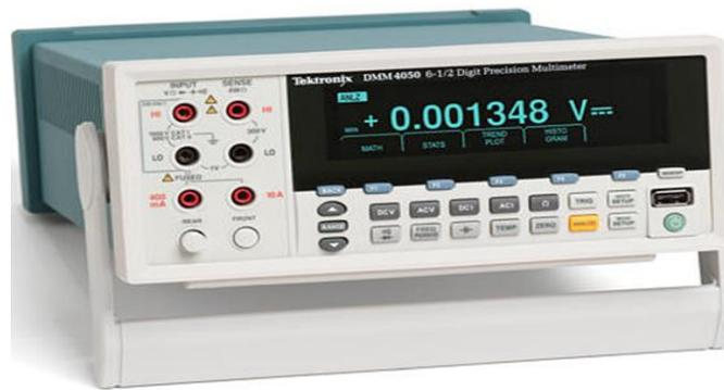
Figure 3.9 Digital Multimeter to measure the in-plane resistance
