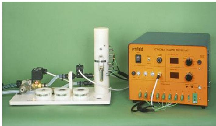
Figure 6.5 Armfield HT11 for Linear Heat Conductivity Measurement
