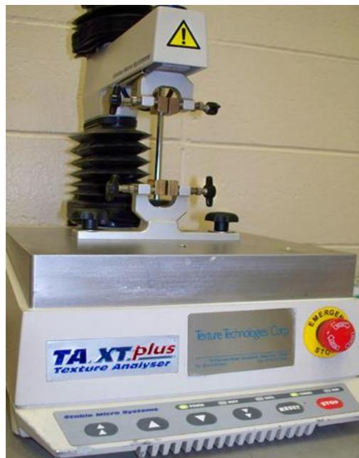
Figure 3.8 Texture analyser to perform Tensile Test
