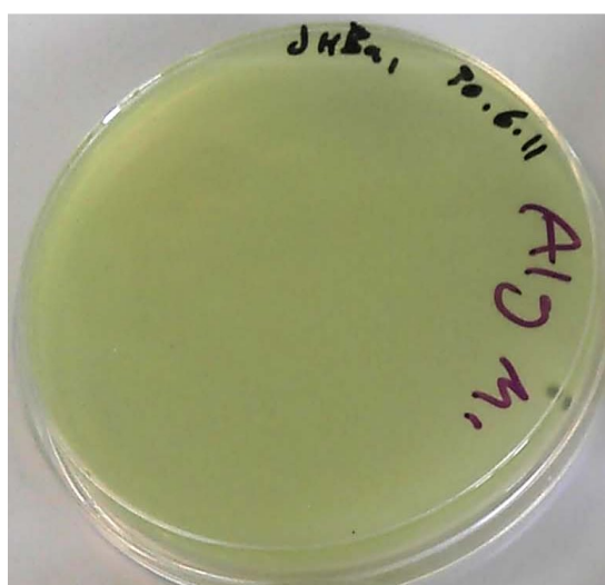
Figure 3-4 Alginate agar plate with no change in colour and no clear zone around the colonies indicative of absence of alginate hydrolysis
