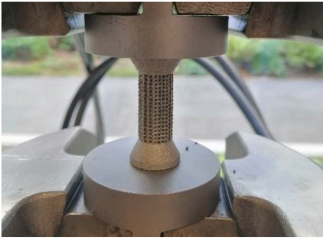
Fig. 3. Photo showing a [001]//LD sample being tested under compression cyclic loading.
